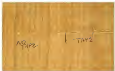
Smooth out a cut. Masking tape significantly reduces the amount of wear-out caused by an aggressive jigsaw cut.
